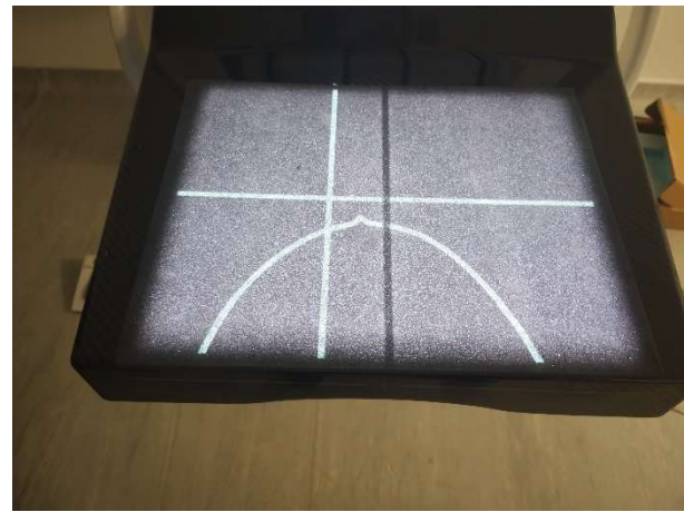
b) The white cross indicating the nipple position fails to find the nipple
