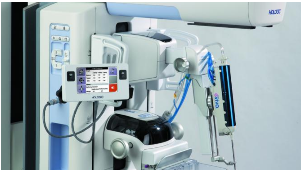
Figure 1. Selenia Dimensions with Affirm biopsy guidance unit and Eviva handpiece
