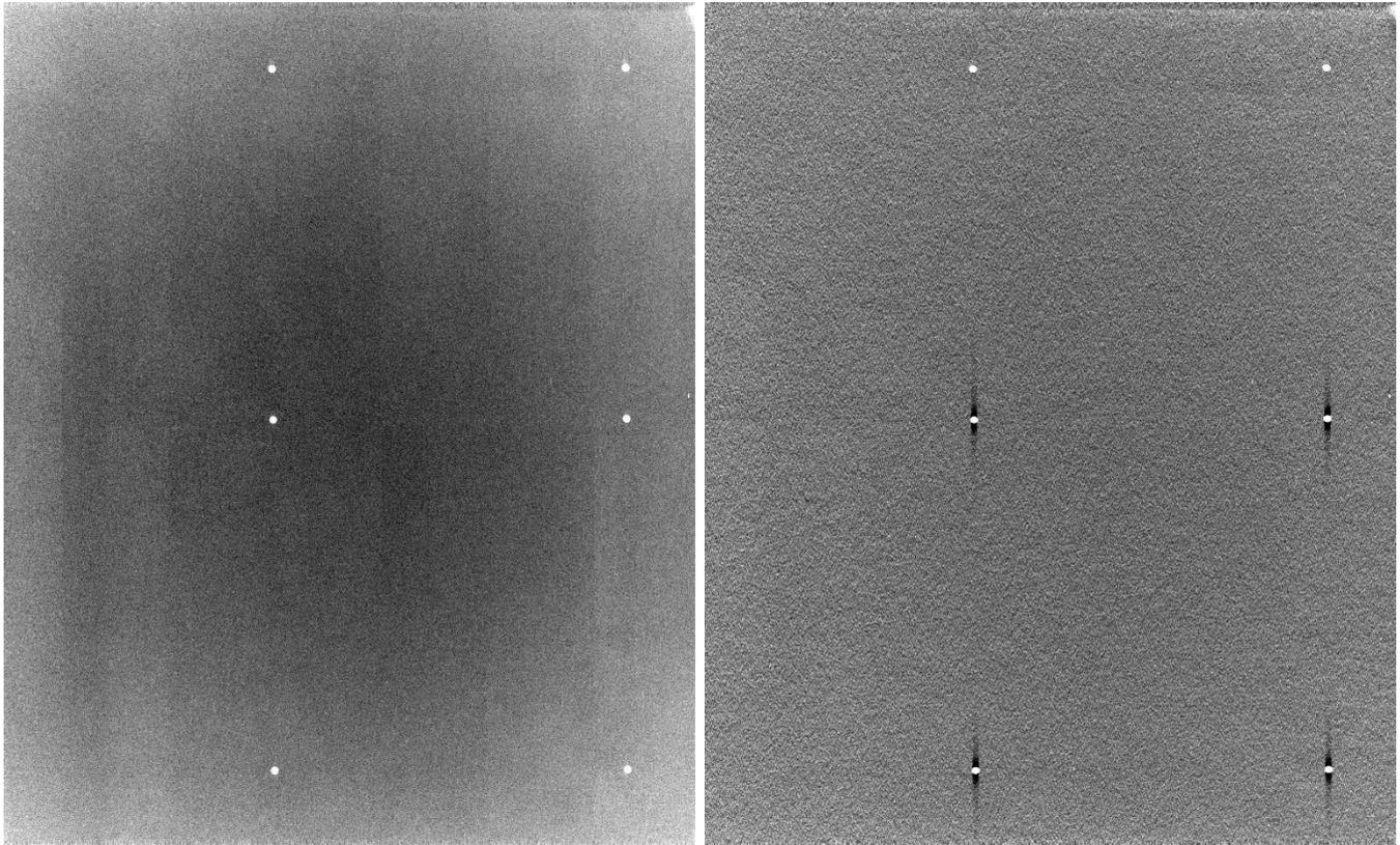
**Figure 11. Appearance in focal plane of best focus of 1mm aluminium ball in 60mm PMMA. QC 'Flatfield tomo' view is on the left, and clinical 'LCC tomo scout' view on the right. The chest wall edge is to the left of each image**
