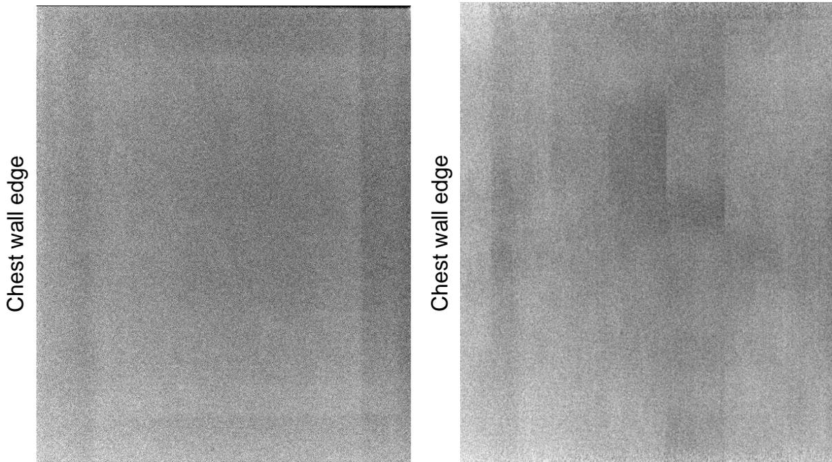
**Figure 14. Images of uniform PMMA: 2D on the left and a tomosynthesis reconstructed focal plane on the right**
