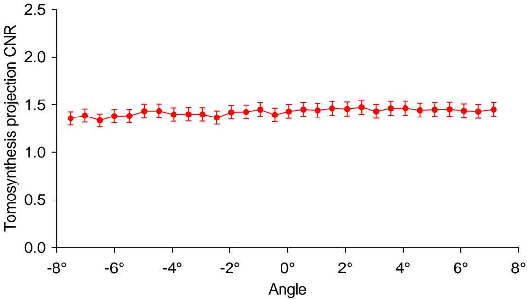
**Figure 6. Variation of CNR with projection angle for a 53mm equivalent breast. Error bars indicate 95% confidence limits.**
