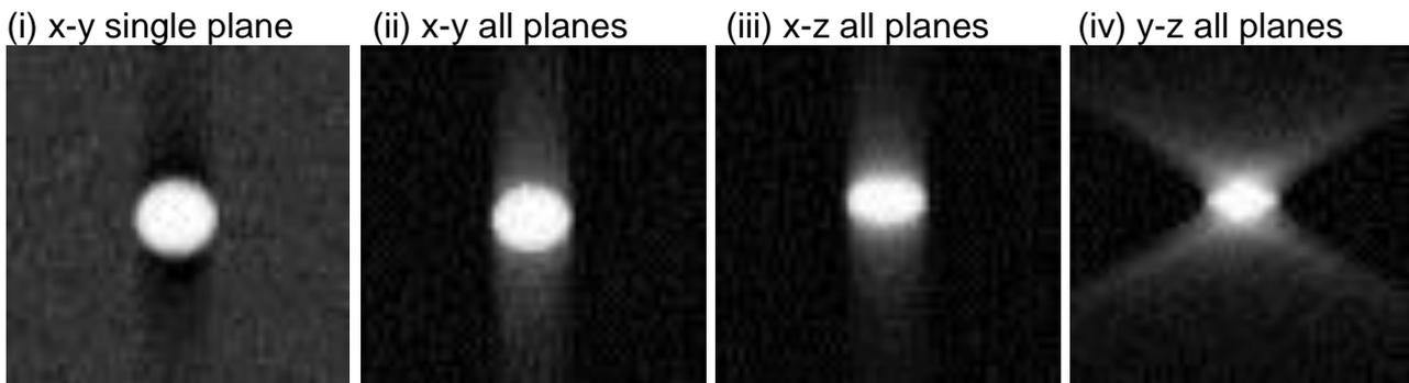
**Figure 13. Extracts from ‘Flatfield tomo’ (top row) and ‘LCC tomo scout’ (bottom row) views showing 1mm aluminium ball in (i) single focal plane, (ii) the maximum intensity projections through all focal planes, and through re-sliced vertical planes in the directions (iii) parallel and (iv) perpendicular to the chest wall.**
