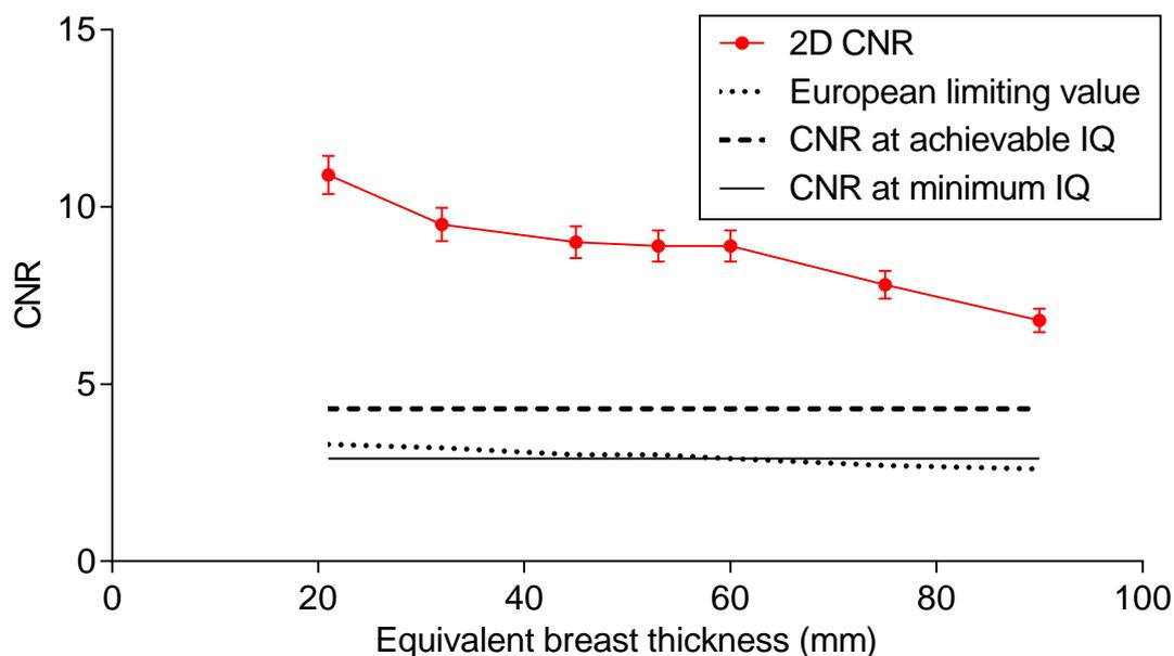
**Figure 4. CNR for 2D images acquired under AEC. Error bars indicate 95% confidence limits.**
