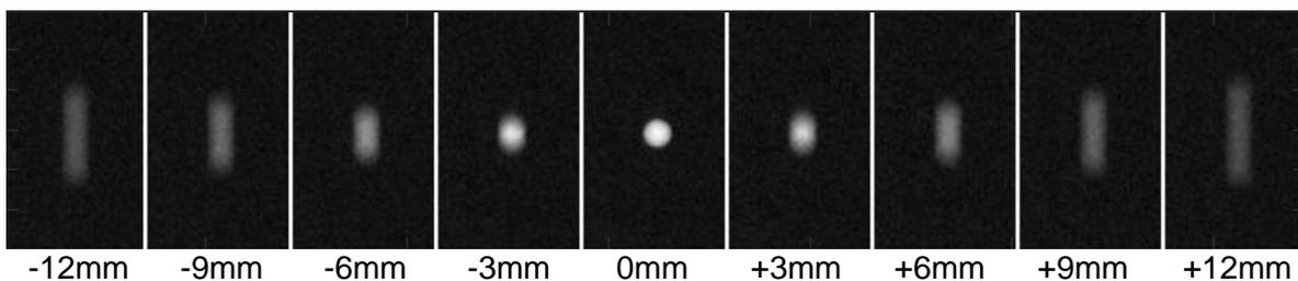
**Figure 12. Appearance of a 1mm aluminium ball in reconstructed focal planes at 3mm intervals extending 12mm either side of the plane of best focus using QC ‘Flatfield tomo’ view**
