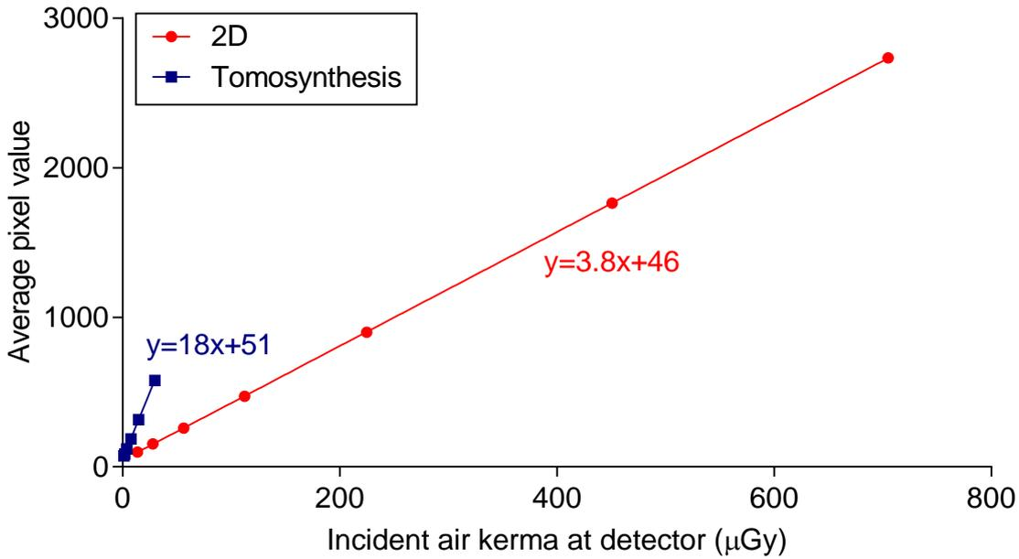
Figure 15. Detector response in 2D and tomosynthesis modes
