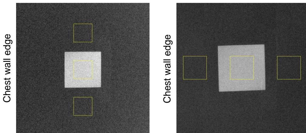
**Figure 2. Location and size of ROI used to determine the CNR in 2D images (left) and tomosynthesis focal planes (right).**
