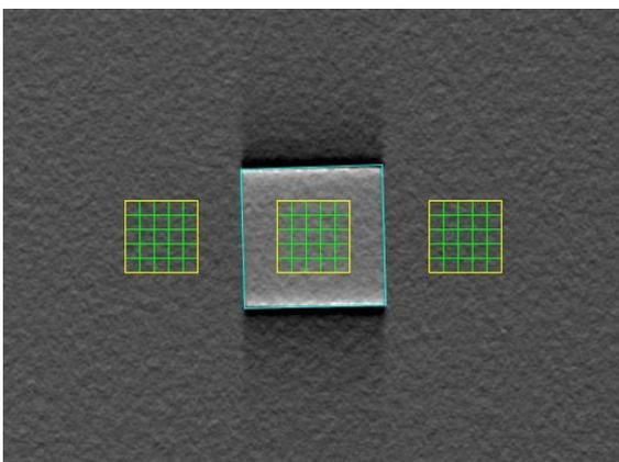
**Figure 3: The position of 5mm x 5mm ROIs for assessment of CNR. (The CWE is to the right)**
